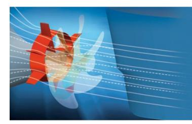
**Stern measures.** While propellers generate powerful thrust, they can also create undesirable swirl which reduces efficiency. Hamburg Süd vessels have been the first to deploy the 'Becker Twisted Fin', an integrated fin system fitted in front of the propeller which produces a counter-swirl in the upstream water flow. This partially cancels out the negative effect of the slipstream swirl, producing energy savings as high as 4%.
